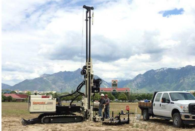
We will require a minimum of 7.0 m length clearance, 4.0 m width clearance and 4.5 - 5.0 m height clearance to drill the wells.
